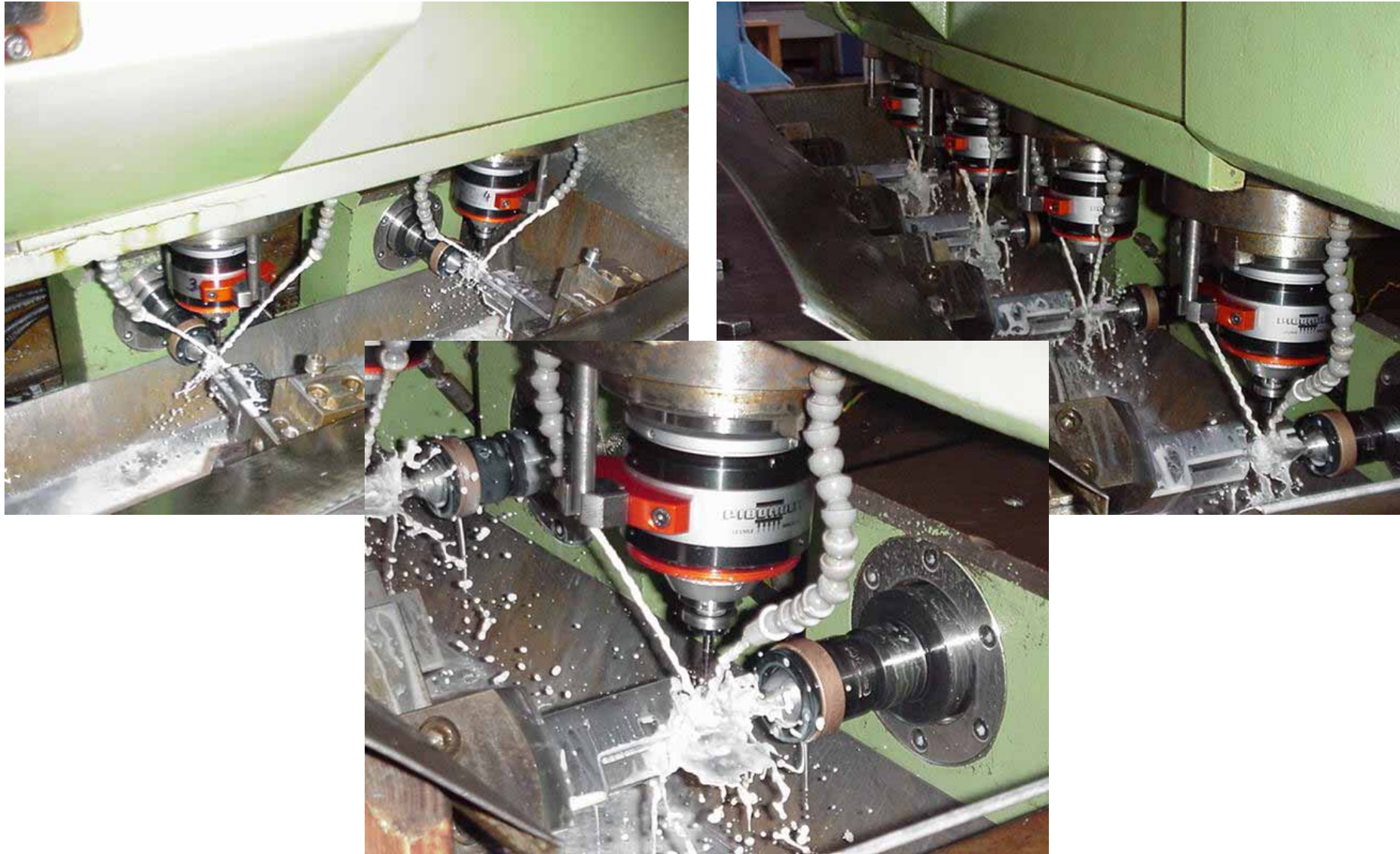
Spindle speeder in machining, 40'000 RPM
