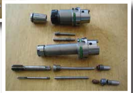
MQL ER-Collet Chuck HSK-A for 2-channel
