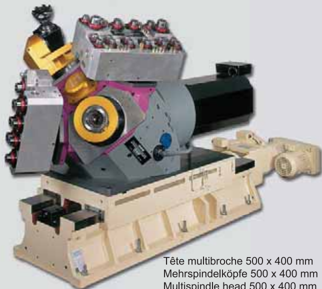
Machine transfert rotatif (TRI 306) Rundtakt-Transfermaschine (TRI 306) Type TRI 306 on Rotary Transfer Machine
